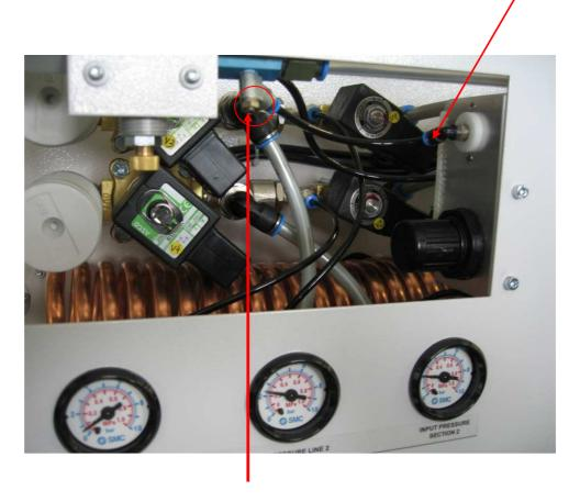
You can set the flow with an internal screw here.
