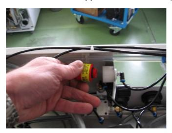
Place the new sensor and tighten it only with hand. The O'ring seal doesn't need more. Connect the electric cord. Be careful with the connector position
