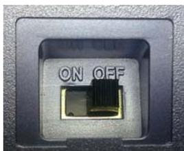
**Figure 5: Slide switch to “OFF” mode after recovery process**
