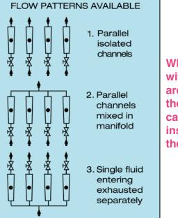
When meters with valves are ordered the valve cartridges are installed at the inlet.
