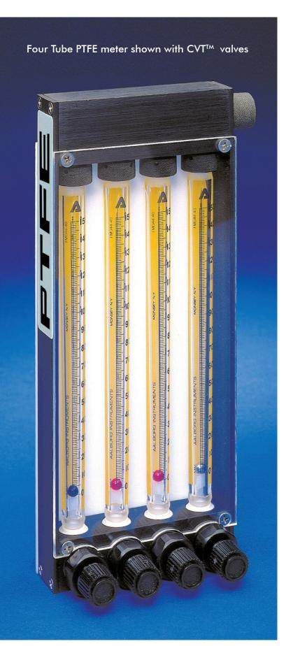
Model Tx Multiple Tube PTFE-Glass Flow meters combine the convenience of multiple tube meters with the unique design features of single tube PTFE-Glass flow meters. These meters are available with the same interchangeable 65mm or 150mm glass flow tubes used in single tube designs and they are available with or without built-in PTFE needle valves.
