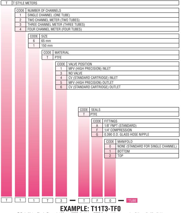
T-Style Meter, Single Channel, 150mm, PTFE, No Valve, PTFE Seals, 1/4" compression fittings, No Manifold.
