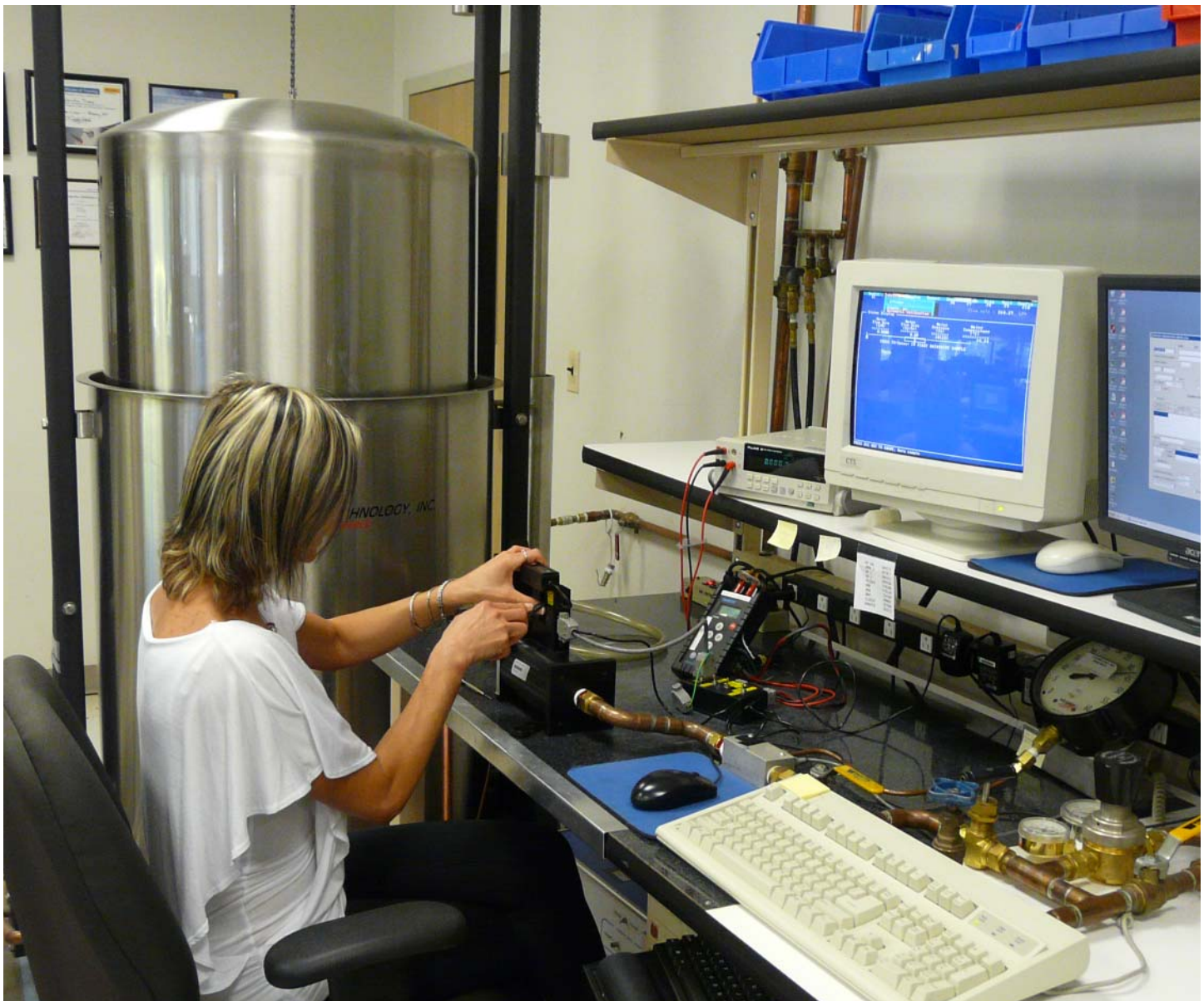
Bell prover used by technician in calibrating high flow capacity flow meter.
